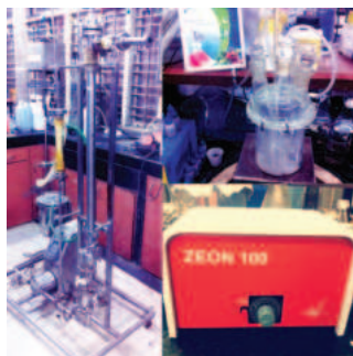
Figure 2: Clockwise: 1. Ultrafiltration Dual Membrane Pilot Plant, 2. Catalytic Ozonation Setup, 3. Zeon 100 - Ozonator
