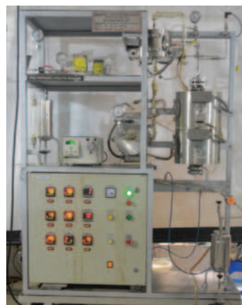
Trickle-bed reactor for production of bio-hydrogenated diesel from non-edible vegetable oil
